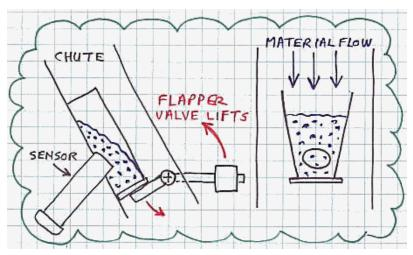
material, when it will open and let the material out. This also prevents the blockages and build-up which could be caused by lumpy material.
