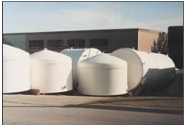
FOOD INDUSTRY: ▶ 12' Diameter / various heights 12 Tanks Steam treated — Cone bottom
