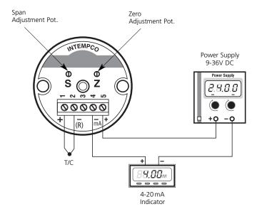
The diagram above represents the connection method to provide the 4-20 mA with a current loop output. The input to the TT810 is either a thermocouple or a thermocouple simulator (Pins 1&2). The output loop (Pins 4&5), the indicator and the transmitter are powered by a 9 to 36 VDC power supply. The indicator could be replaced by a calibrator, controller, a data logger, etc.
