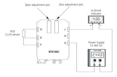
The diagram above represents the connection method to provide the 4-20 mA with a current loop output. In most cases, the RT610Di would take the form of a 3 wire output probe assembly. The output loop, the indicator and the transmitter are powered by a 12 to 36 VDC power supply. The indicator could be replaced by a controller, a data logger, etc.
