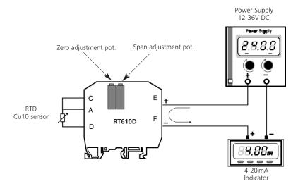
The diagram above represents the connection method to provide the 4-20 mA with a current loop output. In most cases, the RT610D would take the form of a 3 wire output probe assembly. The output loop, the indicator and the transmitter are powered by a 12 to 36 VDC power supply. The indicator could be replaced by a controller, a data logger, etc.
