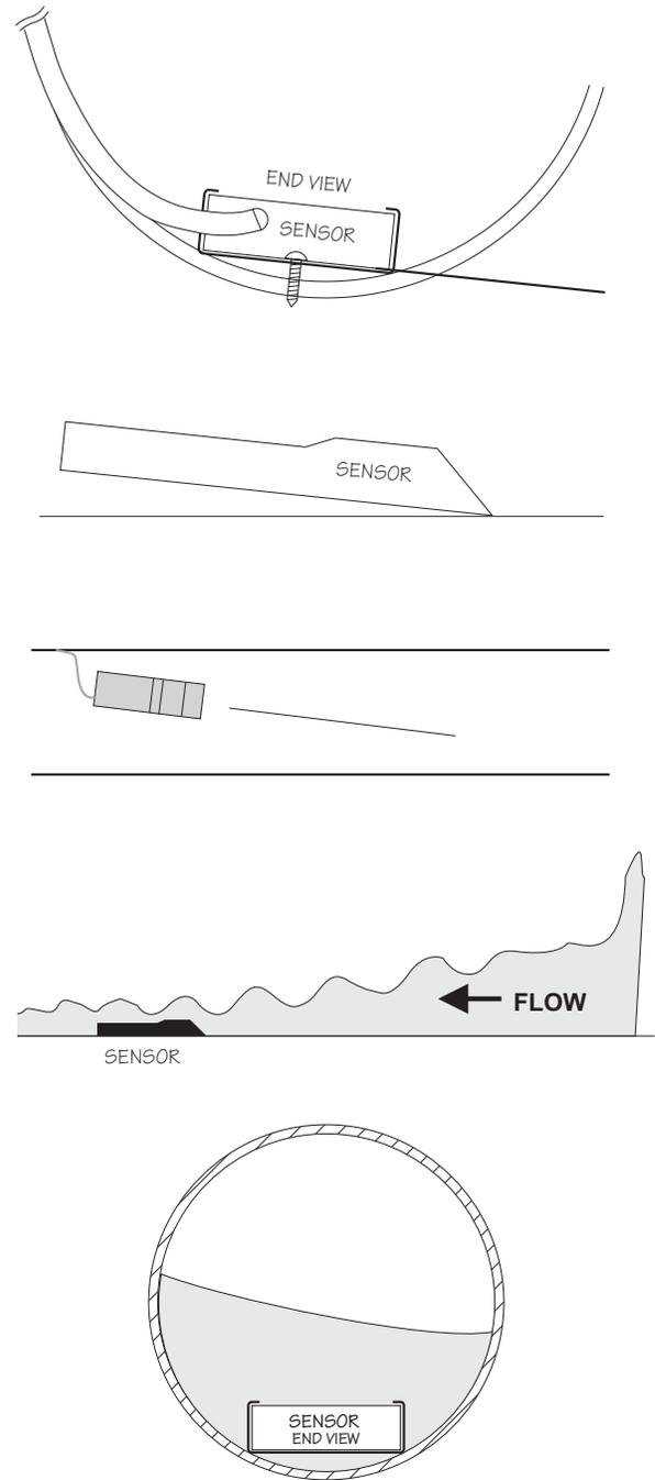
**OPTIONAL PIPE BAND MOUNTING WITH QZ02 SENSOR**
