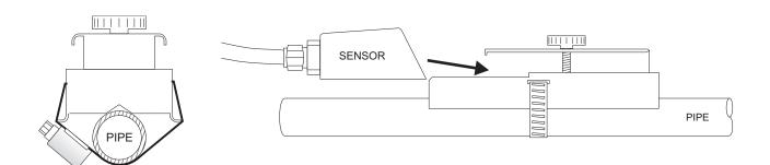
Mount the PC4 pipe clamp as illustrated on pipes 0.6" / 15 mm OD or larger. Stainless steel bands are included for mounting on pipes up to 32" / 81 cm OD.
