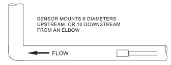
TURBULENCE INCREASING DEVICES: Elbows, flanged connections and tees tend to introduce desirable conditions of an evenly distributed flow profile with some air or gases entrained in the flow. Sensor mounting 6 pipe diameters upstream and 10 diameters downstream from these disturbances is generally optimum.
