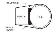
Over time temporary coupling compounds (e.g. Petroleum Gel) may gradually sag away from the sensor resulting in reduced signal
