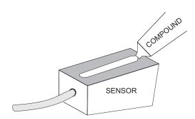
Use the PC4 pipe clamp (supplied) as illustrated above or use a loop of electrical tape for temporary mounting. Apply silicon coupling compound #4 to the coloured face of the sensor. A bead, similar to toothpaste on a toothbrush, is ideal. Do not overtighten (crush the sensor).
