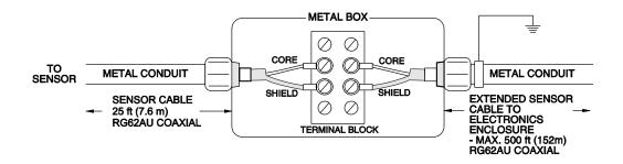
Note: Optional Watertight steel NEMA4 Junction Boxes with terminal strips (Option JB) are available from Greyline Instruments.
