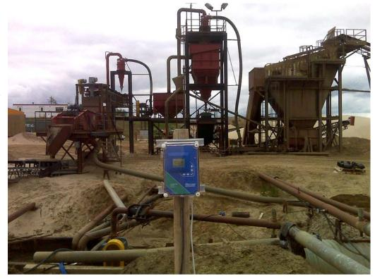
CanFrac produce "fracturing sand" used by the oil and gas industry. This special type of sand is pumped into an oil or gas well to help keep fractures between layers of rock propped open to allow hydrocarbons to flow to the wellbore. CanFrac consulted Tarpon Energy Services of Calgary, Alberta for solutions when their inline flowmeters were damaged by the abrasive sand. Tarpon proposed the Greyline DFM 5.0 Doppler Flowmeter.
