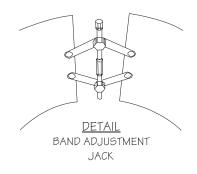
Use optional VSJ stainless steel Half-Pipe Mounting Bands for easy Sensor installation in large round pipes.
