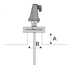
Avoid nozzle size higher than 5.9", especially when B < 3.1".
